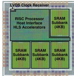
Figure 1. **BRGTC1 Test Chip** – A taped-out  $2 \times 2$  mm 1.3 M-transistor test chip in IBM 130 nm designed and implemented using our new PyMTL hardware modeling framework. Chip includes a simple pipelined 32-bit RISC processor, custom LVDS clock receiver, 16 KB of on-chip SRAM, and application-specific accelerators generated using commercial C-to-RTL high-level synthesis tools.
